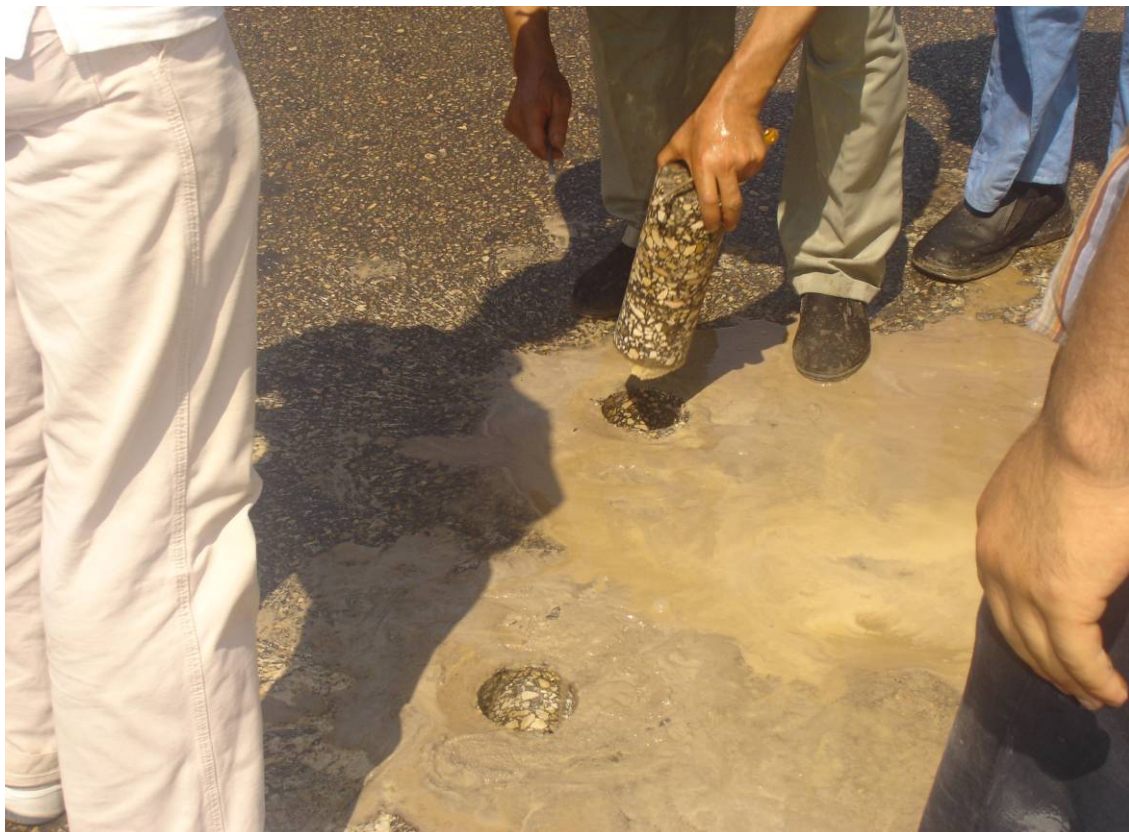
Figure (4-4): Sample of core extraction.
