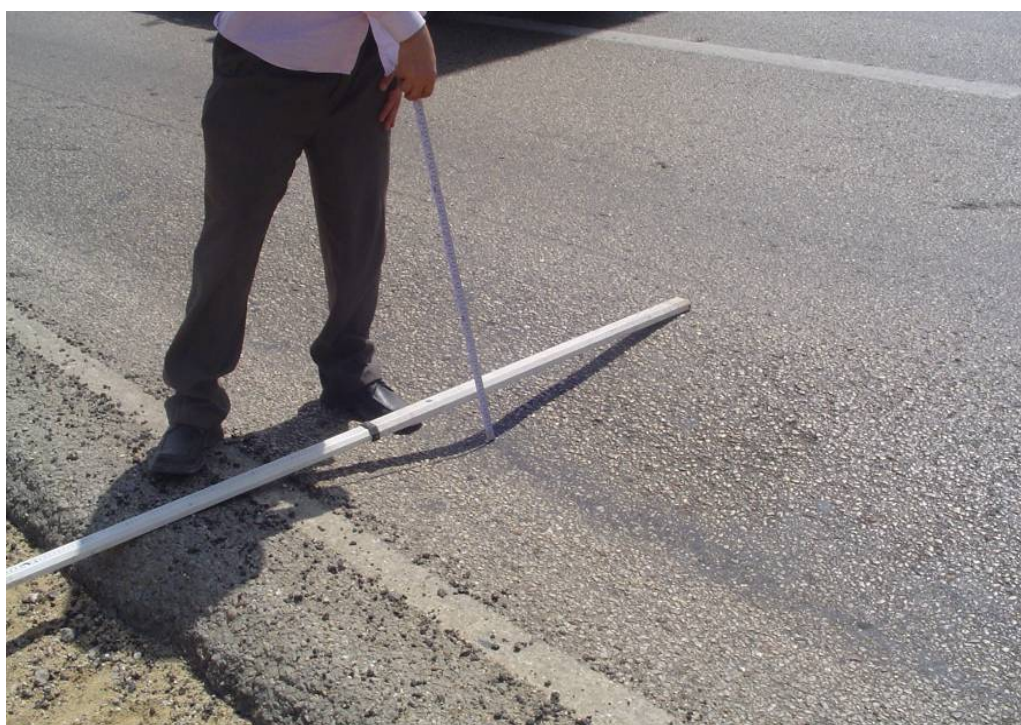
Figure (3-5): Rutting, outer carriageway, (km 41.9).
